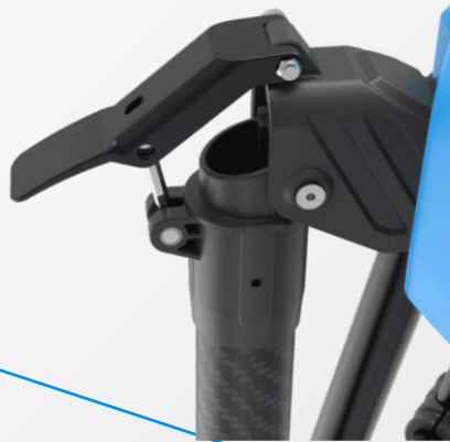
Foldable arm Four link locking
