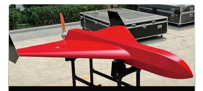
The entire fuselage is made of aviation carbon fiber composite material, with high structural strength and light weight, suitable for various application scenarios such as harsh environments and heavy mission loads
